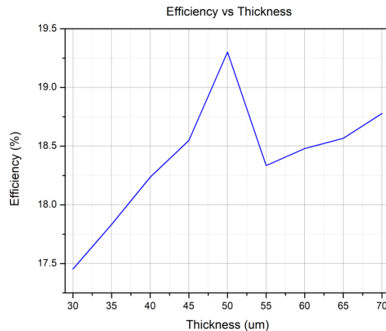
Figure 7. Conversion efficiency for different value of solar cell thickness at bulk concentration 1 \cdot 10^{17} .
