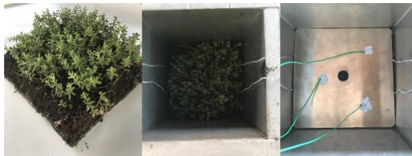
Picture 5: Placing the sample into chamber
