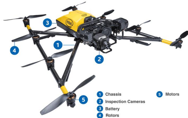
Figure 1: Intel Falcon 8+ Overview. Intel Corporation. Adapted from https://www.intel.com/content/dam/www/public/us/en/images/product/RWD/drones-falcon-8-plus-infographic-overall-16x9.png.rendition.intel.web.978.550.png
