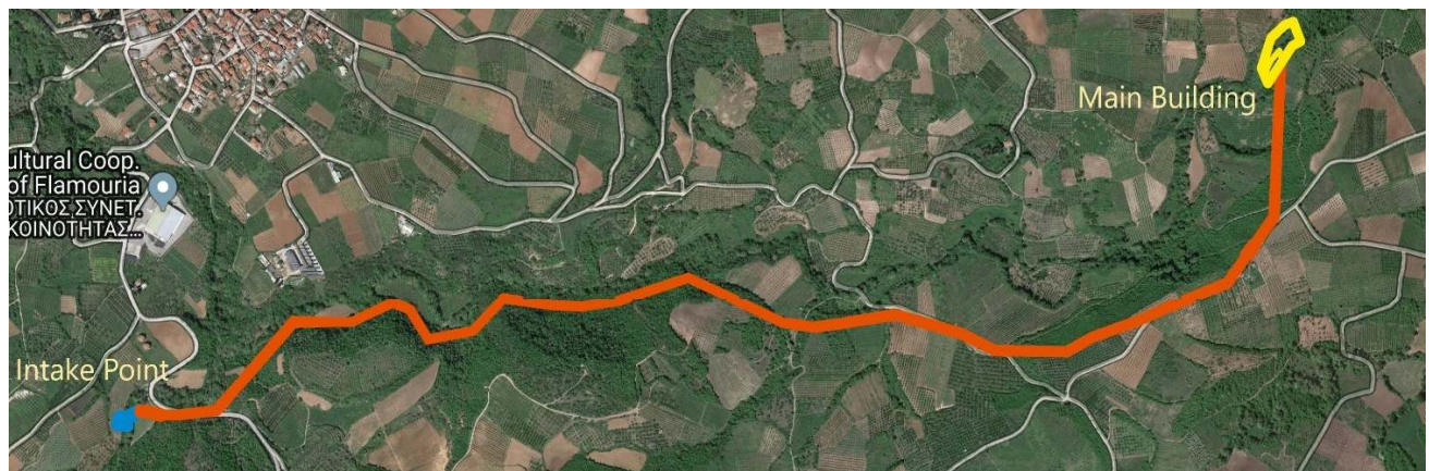
II: Map of the SHP of Flamouria. The intake point (blue), the penstock (orange) and the main building (yellow) are drawn
